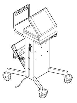
Start by fitting the Cable Management Bar. Unwrap the two fixing screws in the plastic bag attached to the trolley handle. Hold the bar so that the cable notches are uppermost, behind the trolley, and slide the free ends into the grooves beneath the TestBook platform. Holding the bar in position, line up the screw holes in the free ends of the bar with the holes in the trolley body, insert and tighten the fixing screws.
