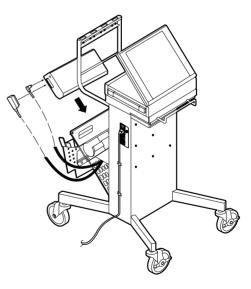
Connect the printer power cable (small connector) and printer interface cable. Note that the power connector should be rotated slightly on insertion to ensure that it goes fully home, and butts firmly against the printer case. Load paper into the printer. The paper feeder on your TestBook printer is designed to handle a stack of dry paper no more than 5mm high. If too much paper is put in, or if the paper is damp, the feeder may jam.
