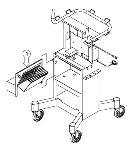
1. Put hinge into securing hole.
