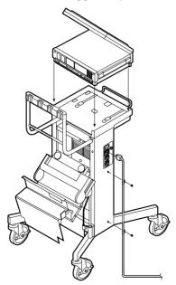
Now look at the back of the trolley and locate the power leads hanging out of the two power transformer units. Plug the right hand lead into the power port at the right rear of the TestBook. The identifying symbol above this port is as shown in the previous section.
