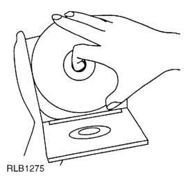
Place the new CD into the caddy so that the labelled side is facing up. The lettering on the CD should be visible through the clear plastic.
