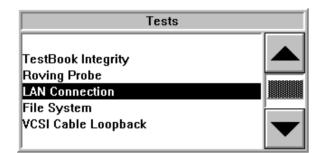
Touch the Integrity Tests button to view the Integrity Tests menu. Use the up and down arrows on the right - hand side of the scroll box to highlight your selection. Then touch Continue on the control panel to run the selected test. A new screen will appear and the test that you selected will begin automatically.
